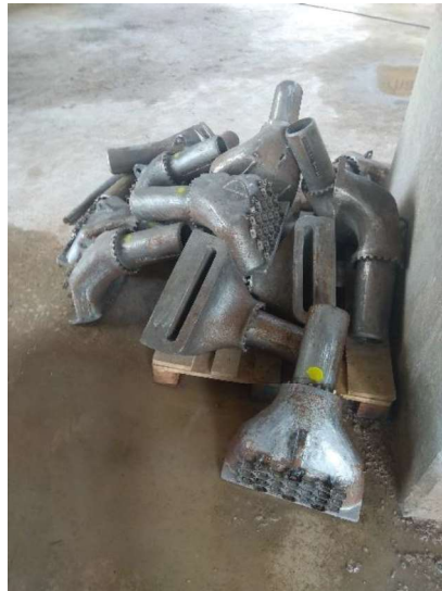
Gambar.13 Nozzle Air blaster 90°
