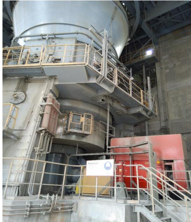
Gambar 1. *Loesche Vertical roller mill*
