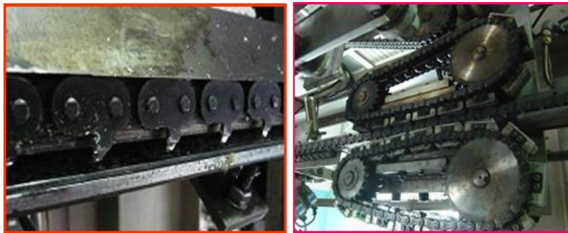
Gambar.8 Spike chain dan caterpillar
